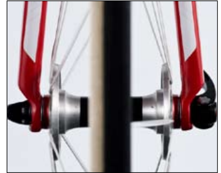
Figure 18. Wide stance of hub flanges, and outboard placement of fork legs relative to the dropouts
